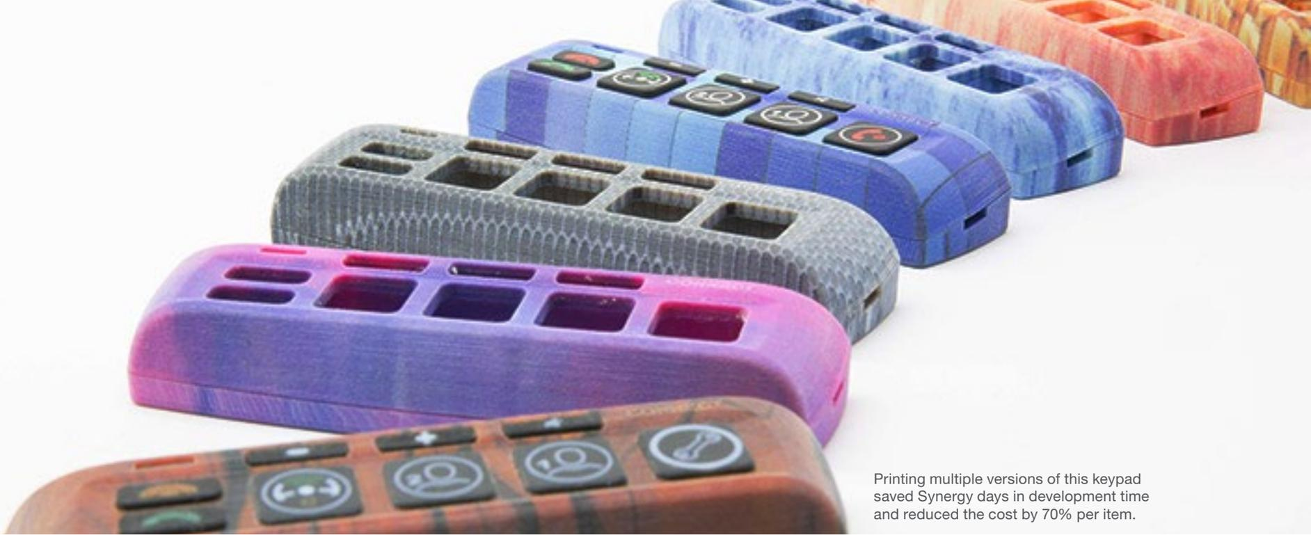
Printing multiple versions of this keypad saved Synergy days in development time and reduced the cost by 70% per item.
