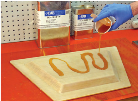
Figure B-4: Pouring epoxy on the tool.
