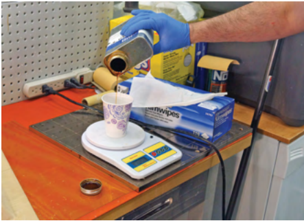
Figure B-2: Weighing the epoxy.
