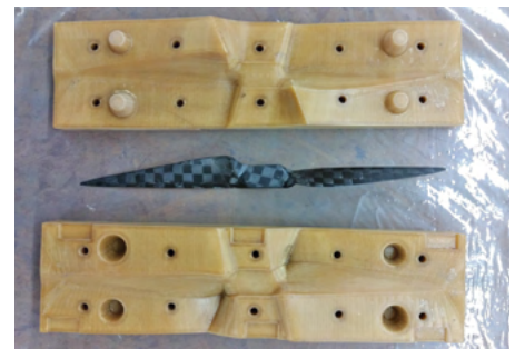
Figure 6-13: Carbon/epoxy composite propeller blade produced on a compression mold tool made from ULTEM 1010 resin.
