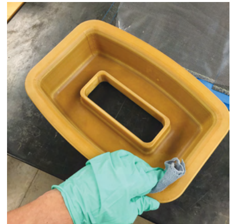
Figure 6-19: UAV bulkhead tool being prepped for use.
