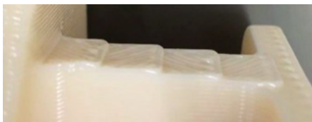
Figure C-7: Stair-stepping with a large slice height.
