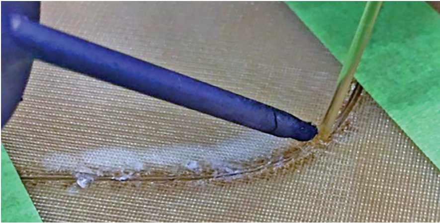
Figure A-5: Filament welding two sections together.
