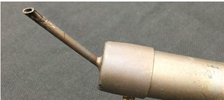
Figure A-2: Soldering nozzle attachment.
