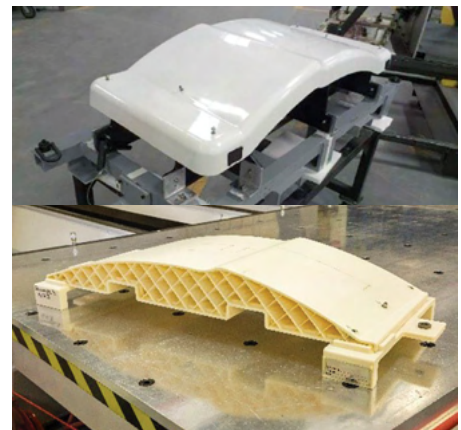
Figure 6-2: Views of the traditions FRP machining fixture (top) and FDM machine fixture (bottom).
