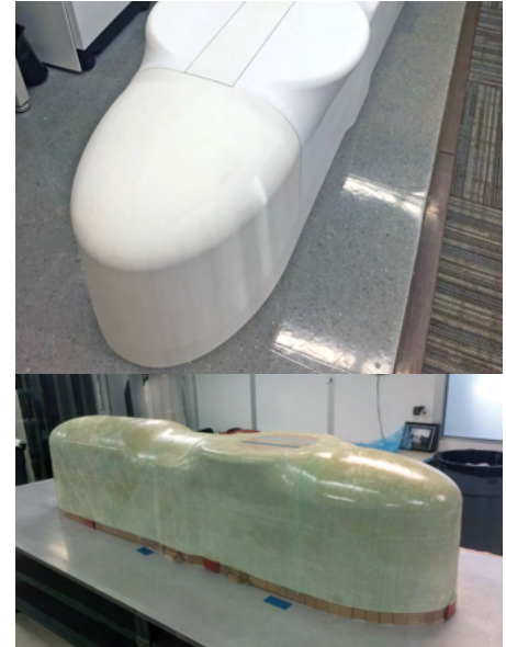
Figure 6-6: Dry fitting the tool after FDM build (top) and tool with cured fiberglass/epoxy fairing (bottom).
