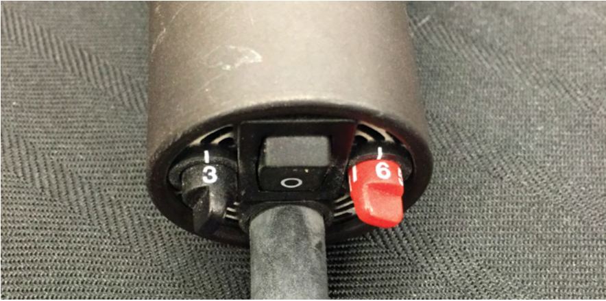
Figure A-3: Fan and temperature settings for ULTEM 1010 resin if using a Leister Hot Jet S hot-air hand tool.
