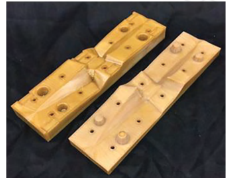
Figure 6-12: Propeller compression molding tool: horizontal build orientation (top), matched mold halves (bottom).
