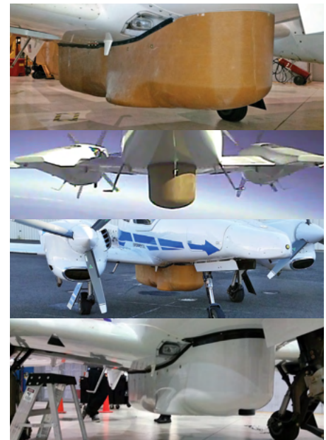
Figure 6-7: Composite belly pod fairing installed on Centaur aircraft (before and after painting).
