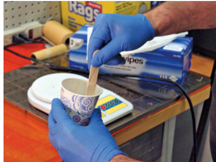
Figure B-3: Mixing the epoxy.
