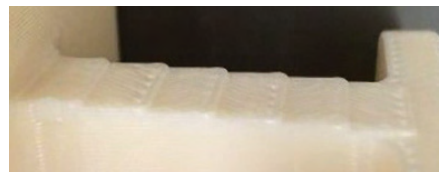
Figure C-8: Stair-stepping with a small slice height.
