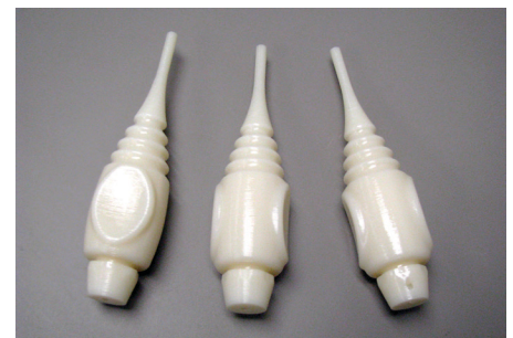
Figure 15: ABS is preferred for patterns because it is easy to finish and low cost.
