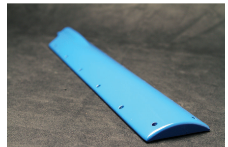
Figure 22: An FDM pattern (painted) can be used to create multiple molds.
