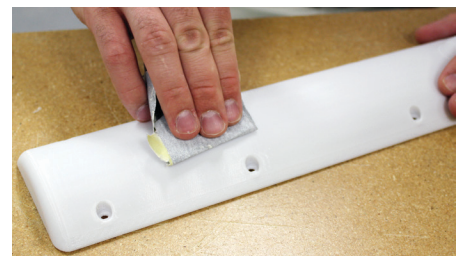
Figure 19: Sand pattern after support removal.
