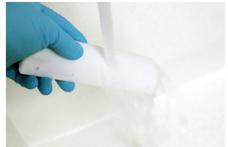
Figure 18: Thoroughly wash pattern to remove support removal detergent.
