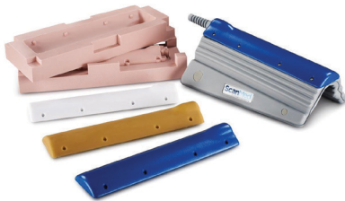
Silicone molded MRI cover and tooling. Clockwise from top left, silicone mold, complete MRI assembly with cast urethane cover, finished and painted urethane cover, raw cast urethane cover, FDM master pattern for creating the silicone mold.
