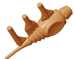
Figure 7: Gates and vents are added to the CAD model of the pattern.
