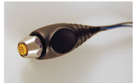
Figure 2: Overmolded connector that was cast in an RTV mold made from an FDM pattern.
