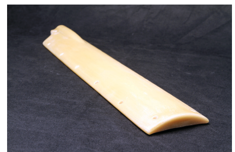
Figure 23: A urethane casting before painting.
