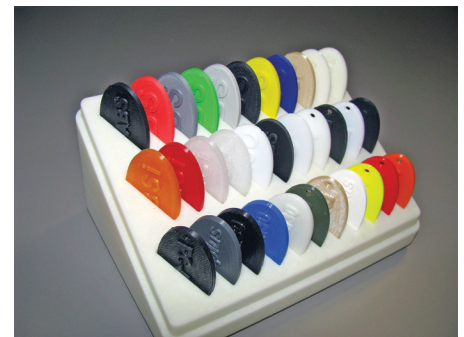
Figure 14: All FDM materials are suitable for RTV patterns.
