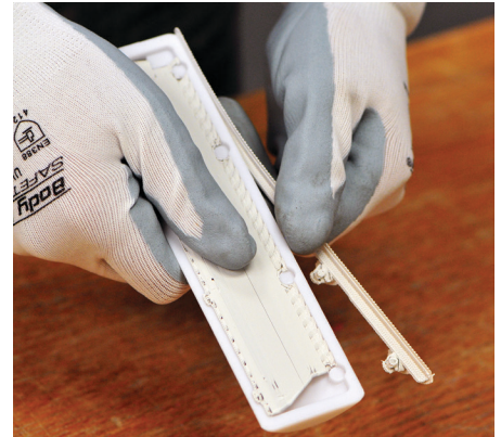
Figure 16: Remove breakaway support material.
