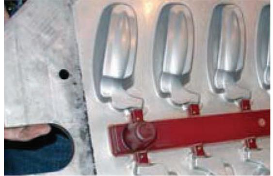
Figure 2: Machined aluminum matchplate.
