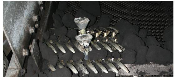
Figure 5: Vibratory bed for sand removal.
