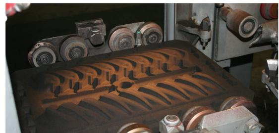
Figure 31: Cope side of sand mold for window handle.
