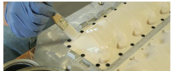
Figure 28: Apply a top coat to seal pores and provide added abrasion resistance.
