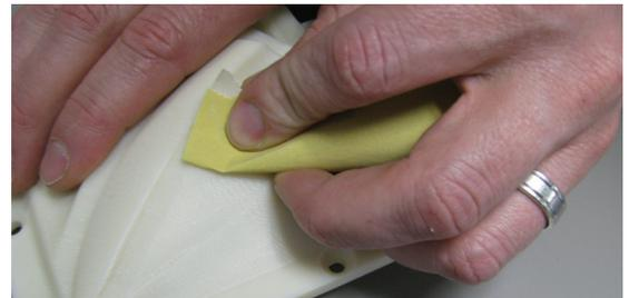
Figure 25: After support removal, smooth pattern surfaces.
