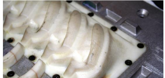
Figure 26: Mount (bolt) FDM insert to machined matchplate blank.
