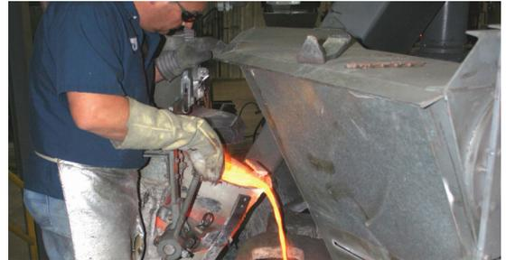
Figure 4: Casting metal into green sand mold.
