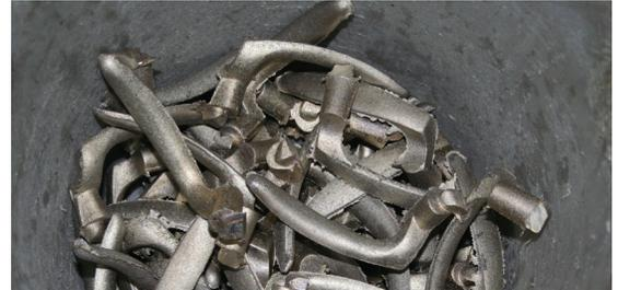
Figure 36: Raw window handle castings ready for finishing.
