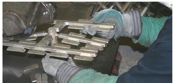
Figure 35: Cut off gates.
