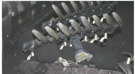
Figure 34: Break out castings from sand mold.
