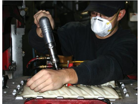
Figure 29: Mount matchplate in automated molding machine.
