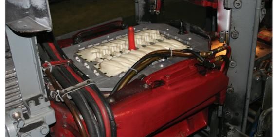
Figure 30: Matchplate in automated molding machine.
