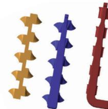
Figure 14: CAD models of interchangeable runner systems for casting refinement.
