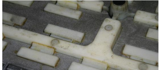
Figure 15: Making gating and runner system as a separate piece; it may be interchanged with alternate configurations.
