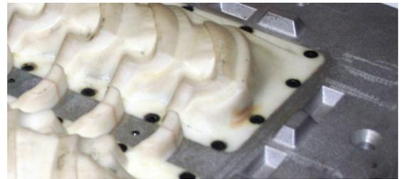
Figure 12: Matchplate blank incorporates a thick “rib” between inserts for stiffening.
