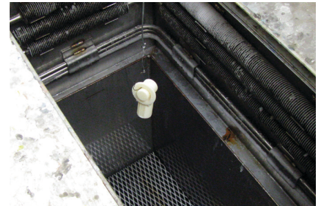
Figure 11: Finishing Touch Smoothing Station seals and smooths patterns in a few seconds.
