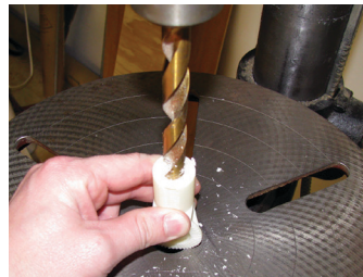
Figure 16: Drill through the outer shell of the pattern at the gate location.
