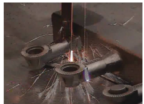
Figure 24: Cut off gates from cast parts.
