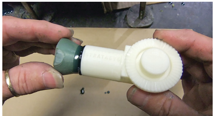
Figure 18: Wax-weld gates and vents to the FDM pattern.
