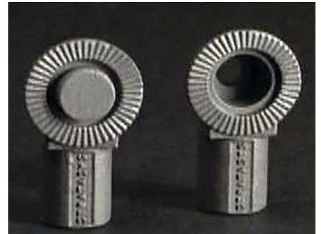
Figure 27: Gear set castings produced from FDM patterns.
