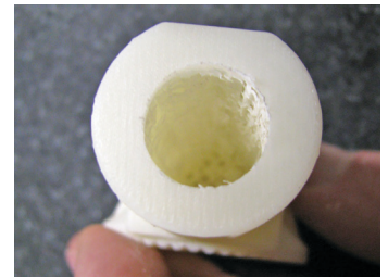
Figure 17: The hole, which will be covered by a wax gate, exposes the sparse fill to high temperatures early in the furnace cycle.
