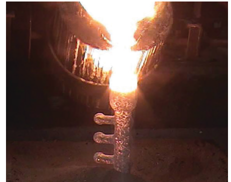
Figure 3: Pouring molten metal into ceramic shell.
