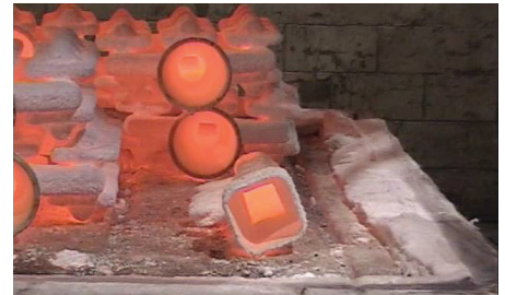
Figure 22: Pre-heat ceramic shell prior to pouring metal.
