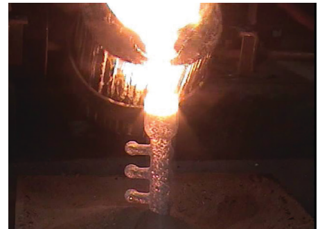
Figure 23: Cast metal into shell.
