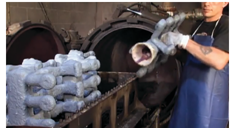
Figure 20: Begin the burnout process with a de-waxing step (autoclave shown).
