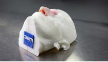
Figure 13: Consumable models like the nasal cavity (top) can be placed in a reusable fixture (head model, bottom).
