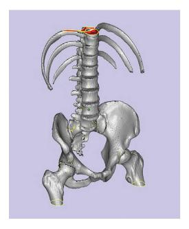
10.3.4. The file is still just a shell so bring it into the Fix Wizard and run automatic fixes by clicking Follow Advice on the part until it is a solid body without any overlapping surfaces. This will require about six automatic fixes.
