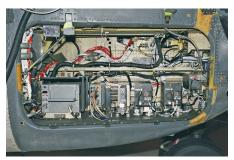
Figure 2: Super Stallion's avionics bay houses high-value, closely packed components with complex routing paths.
