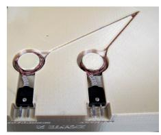
Figure 15: Place and bond sensors or RFID tags in FDM surrogate.
