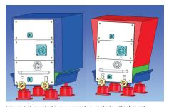
Figure 6: For interface surrogates, include attachment hardware in the CAD model.
