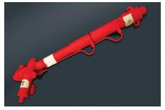
Figure 12: Use colored FDM materials to flag surrogates, such as "Red – remove before delivery."
