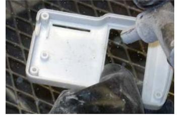
Figure 2: Lightly bead blast all surfaces with a constant, sweeping motion.
