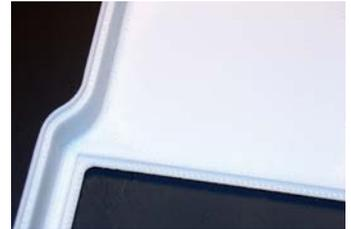
Figure 3: Finished FDM part after only a few minutes of bead blasting.
