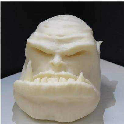
The 3D printed creature after support is removed.
