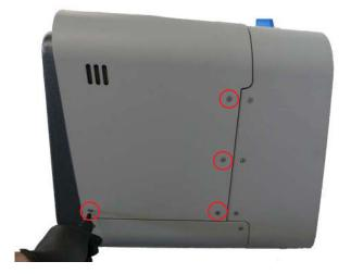
Use a 2.5 mm hex key to unscrew the four screws on the left side of the top shell. Set the screws aside.
