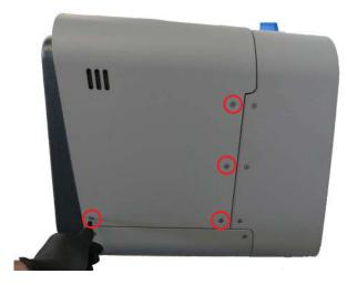
Use a 2.5 mm hex key to reinstall the four screws on the left side of the top shell. Tighten until snug.
