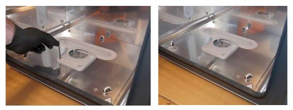
If you have replaced the bottom LED module, reinstall the turntable shroud. Thread the four screws into their screw holes and tighten with the 2.5 mm hex driver until finger tight.
