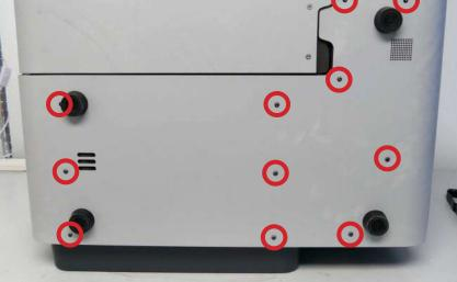
Thread one 2.5 mm flat head hex screw into each of the screw holes in the left and right side of the bottom shell. Thread one 2.5 mm button head hex screw into each of the screw holes in the bottom of the machine. Using a 2.5 mm hex driver, tighten the screws until finger tight.
