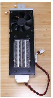
The Stratasys ProLight has two heater modules that heat printed parts during post-curing. If either heater module is malfunctioning or broken, printed parts may not post-cure properly and may not reach their optimal mechanical properties.
