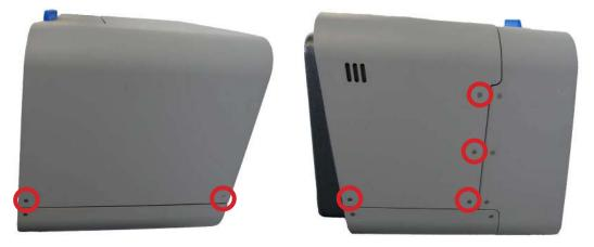
The top shell is secured to the frame of the machine with six hex screws. When facing the front of the Stratasys ProLight, two screws are located on the right side and four are located on the left. Use a 2.5 mm hex driver to unscrew and remove the screws.
