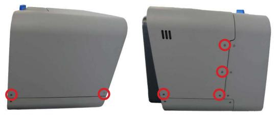
The top shell is secured to the frame of the machine with six hex screws. When facing the front of the Stratasys ProLight, two screws are located on the right side and four are located on the left. Use a 2.5 mm hex driver to unscrew and remove the screws.
