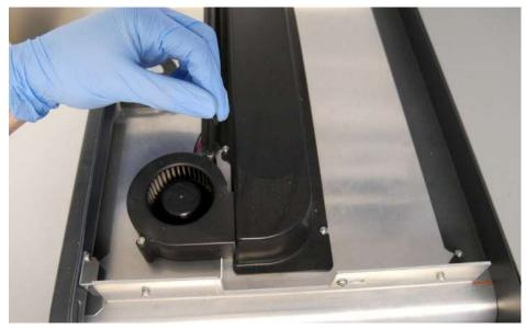
Reinstall the retention screw or screws and tighten with a 2.5 mm hex driver until finger tight.
