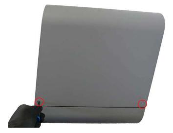
Use a 2.5 mm hex key to unscrew the two screws on the right side of the top shell. Set the screws aside.
