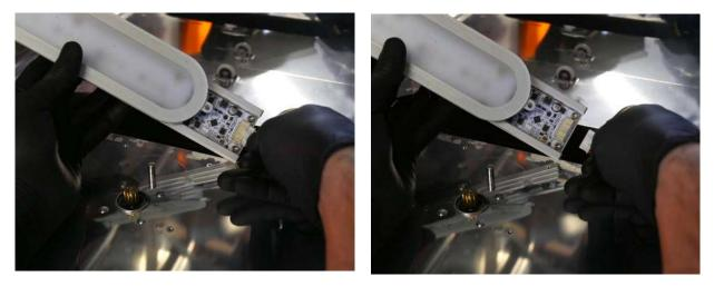
Unplug the LED module cable. When disconnecting the cable, grip the connector, press in on the tab, and separate it from the LED module. Do not pull on the wires themselves.
