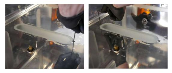
Each LED module is secured by two screws, one on each end. Using the 2.5 mm hex driver, loosen and remove the two screws. If you are replacing the top or left-hand LED module, support the module to keep it from shifting or falling. Set the screws aside.
