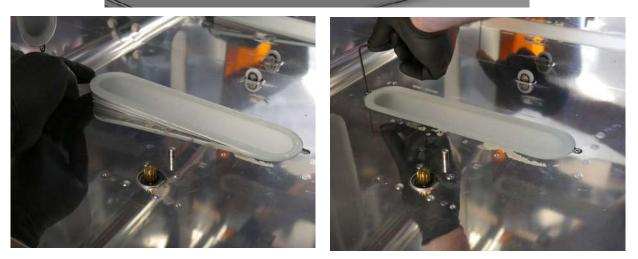
Tilt the LED module back into place. Ensure that the LED module cable is not pinched between the module and the post-cure chamber wall. Thread the two screws into their respective holes. Use the 2.5 mm hex drive to tighten both screws until finger tight.
