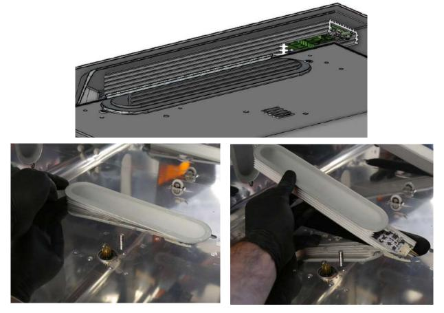
Tilt the LED module away from the body of the Stratasys ProLight. Note that a portion of the LED module extends behind the wall of the post-cure chamber. Do not pull the LED module directly away from the chamber wall.
