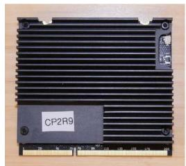
Reinstall the heatsink onto the SOM, making sure the thermal pad on the bottom of the heatsink covers the processor (the largest chip on the board, labeled U6). Ensure that the cutout on the edge of the heatsink allows access to the Wi-Fi antenna port and that the screw holes in the heatsink align with the holes in the SOM.
