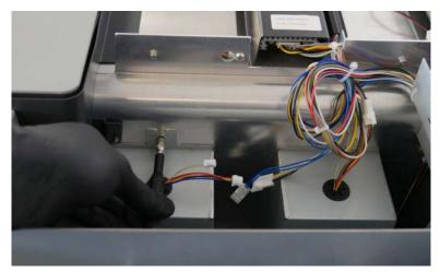
Reinstall the retention nut and tighten it with the 5.5 mm socket driver until finger tight. When installed correctly, the rear heater assembly shroud sits flush against the cure chamber wall.
