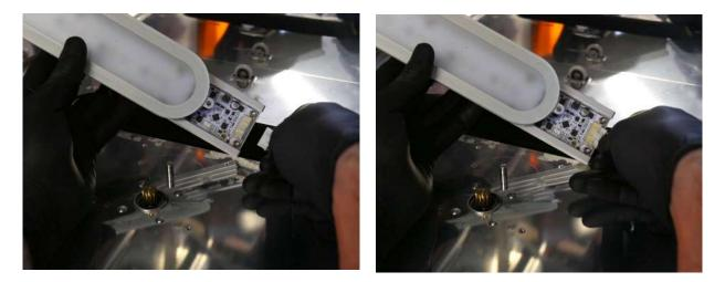
Reconnect the LED module cable. The connector will only plug into the module properly in the correct orientation. Be careful not to bend the pins in the connector.
