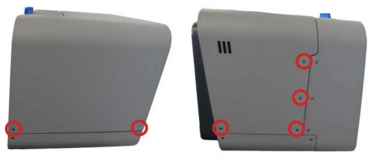
Thread one 2.5 mm hex screw into each of the six screw holes in the top shell. Using a 2.5 mm hex driver, tighten the screws until finger tight.
