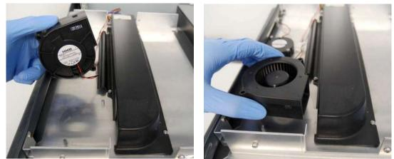
STEP 1: MOUNT AND SECURE THE REPLACEMENT COOLING FAN
