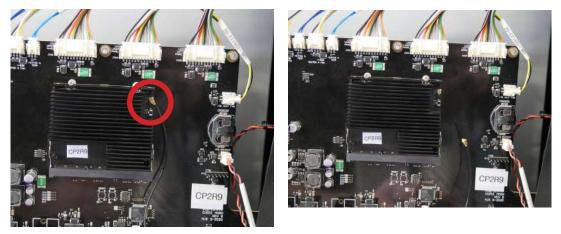
The Wi-Fi antenna is plugged into the SOM at the top-right corner of the board. The connector is accessible through a cutout in the heatsink. Grip the antenna's connector by its housing and disconnect it from the SOM. Do not pull on the antenna itself.
