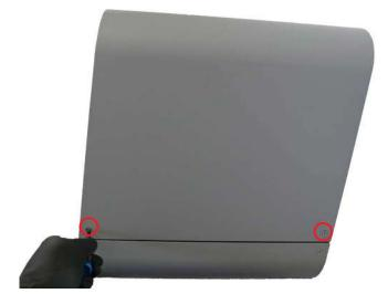
Use a 2.5 mm hex key to reinstall the two screws on the right side of the top shell. Tighten until snug.
