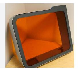
The Stratasys ProLight has a door that helps insulate the machine and contain the light from the LED modules. If the door is damaged, the Stratasys ProLight may not reach or maintain its target temperature. If the door cannot fully close, the machine does not allow you to start a post-curing cycle.
