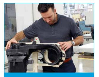
In less than a week, MAHLE had a redesigned, dimensionally accurate and stable part delivered to them from across the world – a process that would have taken 4 to 5 weeks with conventional manufacturing. Thanks to part consolidation, the fixture had a continuous and smooth mating interface, which could only be replicated in a metal fixture at a considerable cost, saving MAHLE thousands by using 3D printing instead of CNC machining.
