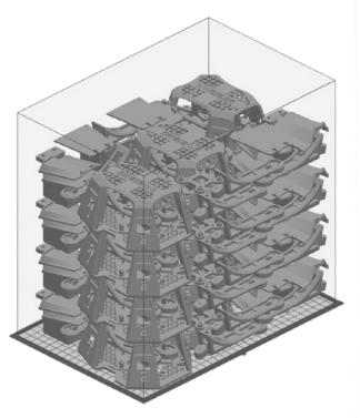
One Stratasys SAF H350 printer can produce 24 drones in a 24-hour period.
