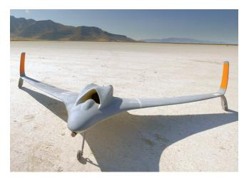
Final 3D printed jet-powered aircraft.
