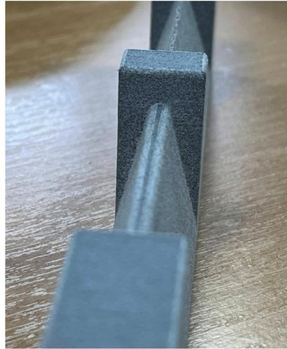
The same effect can also be observed on square edges of up facing material. The slight meniscus lip around the edge can become damaged and look untidy, Figure 6. Adding a very small radius (1mm) to these square edges can mitigate the lipping and reduce damage during depowdering. This approach avoids having to reorient the part in the nest which could compromise aesthetics.
