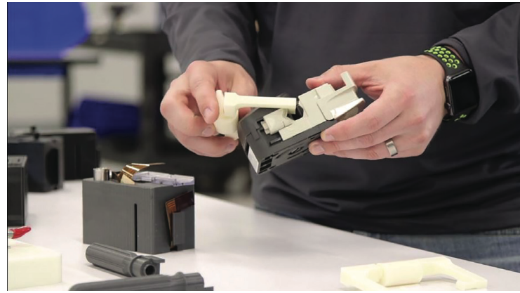
Several of CSI’s 3D printed manufacturing aids
