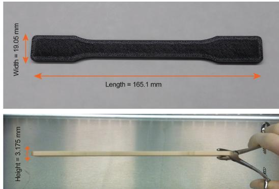
Figure 1: Sample dimensions, (a) Top view (b) Side view
