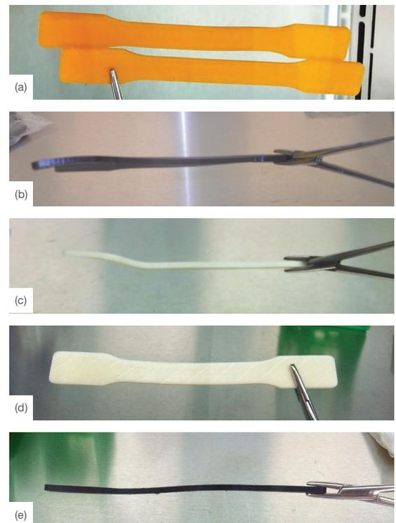
Figure 5: Material changes caused by autoclave, (a) ABSi: bending and multi-sample attachment, (b) ABS-ESD7: bending and multi-sample attachment, (c) ABS-M30: bending, (d) ABS-M30i: bending and indentations, (e) PC-ABS: bending
