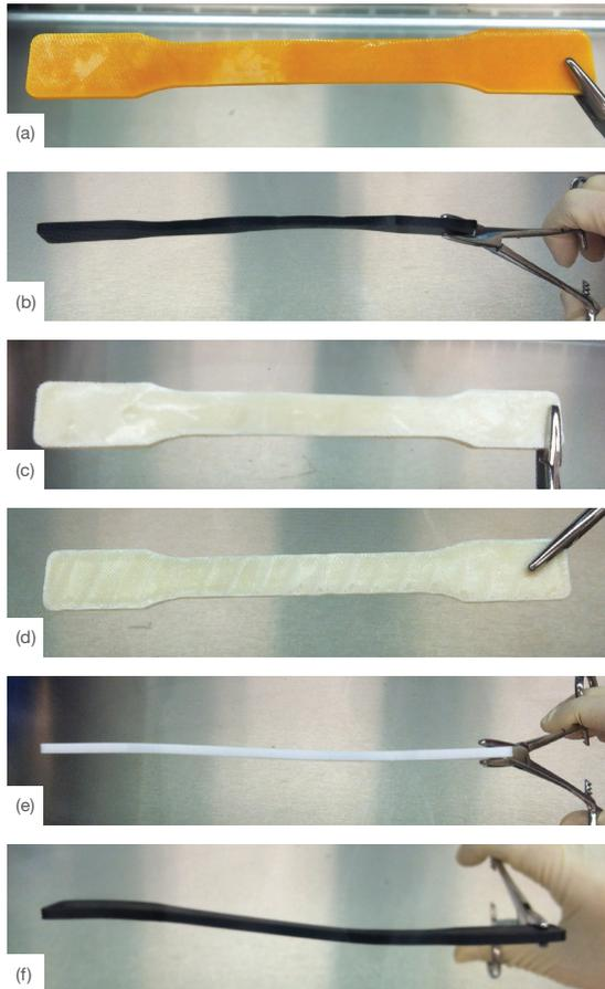
Figure 6: Material changes caused by flash autoclave, (a) ABSi: bending and color change, (b) ABS-ESD7: bending, (c) ABS-M30: bending and indentations, (d) ABS-M30: bending and indentations, (e) PC: bending, (f) PC-ABS: bending
