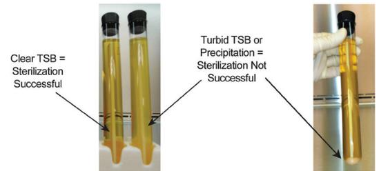
Figure 3: Determining success of sterilization procedure
