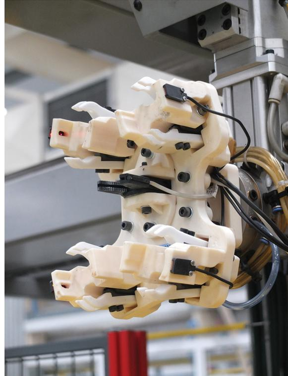
3D printed handling tool for robotic arms enables complex geometries not achievable with CNC.
