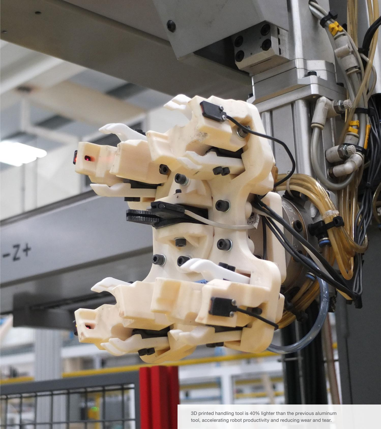
3D printed handling tool is 40% lighter than the previous aluminum tool, accelerating robot productivity and reducing wear and tear.
