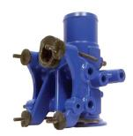
3D printed prototypes attached to a steel part for verification
