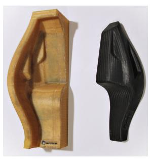
3D printed composite layup tool produced in ULTEM $^{\text{TM}}$  9085 resin, alongside the final carbon-fiber part for use in Formula One racing.
