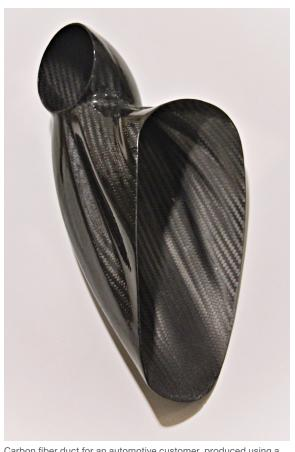
Carbon fiber duct for an automotive customer, produced using a 3D printed sacrificial tool in ST-130 soluble material.
