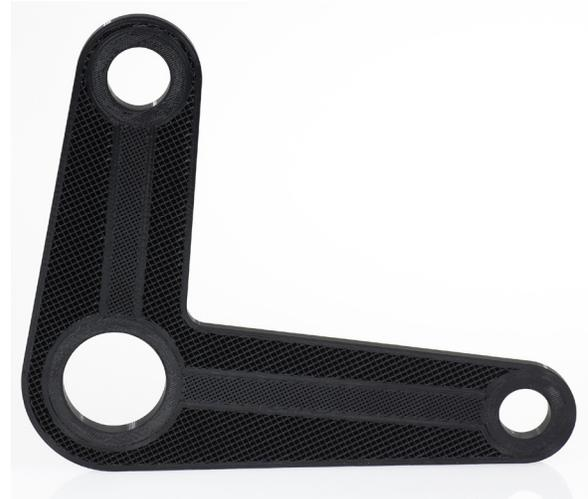
Figure 2-15: Printed bell crank example with multiple infill patterns.
