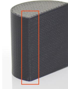
Figure 2-11: Seam placement on edge.
