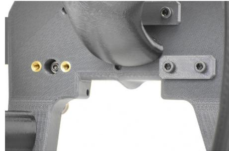
Figure 2-22 Fixture utilizing brass heat set.
