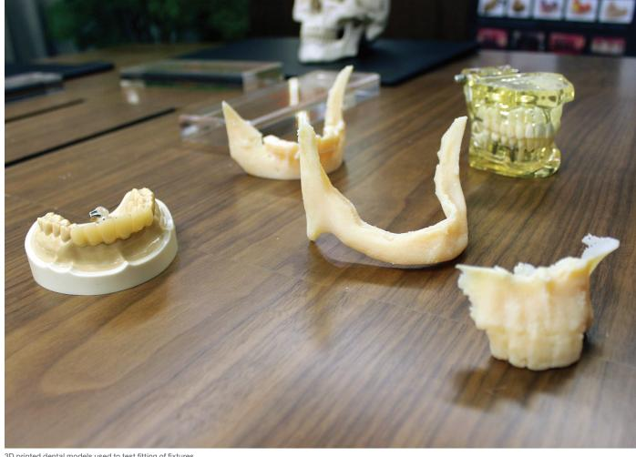
3D printed dental models used to test fitting of fixtures
