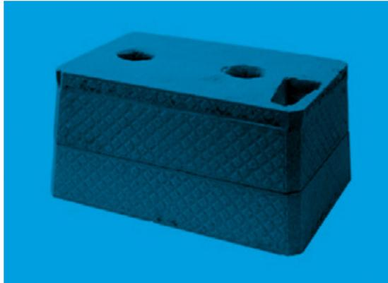
Figure 4: The pattern is removed from the mold
