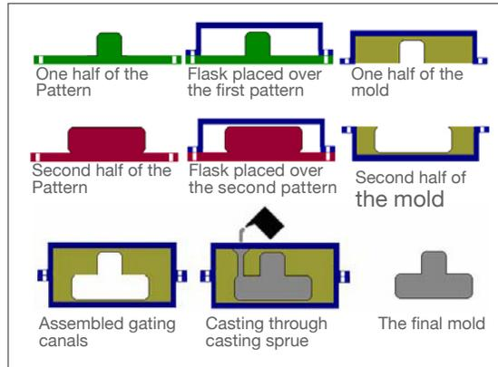
Figure 1: Workflow of the sand casting process
