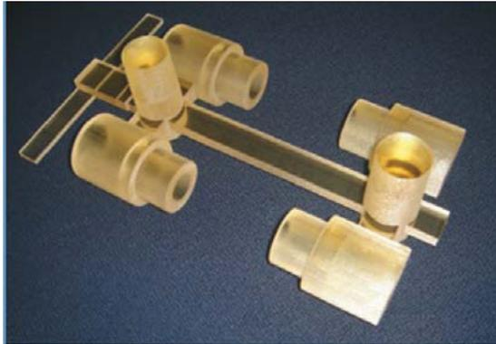
Figure 2: A 3D printed model using PolyJet Technology.
