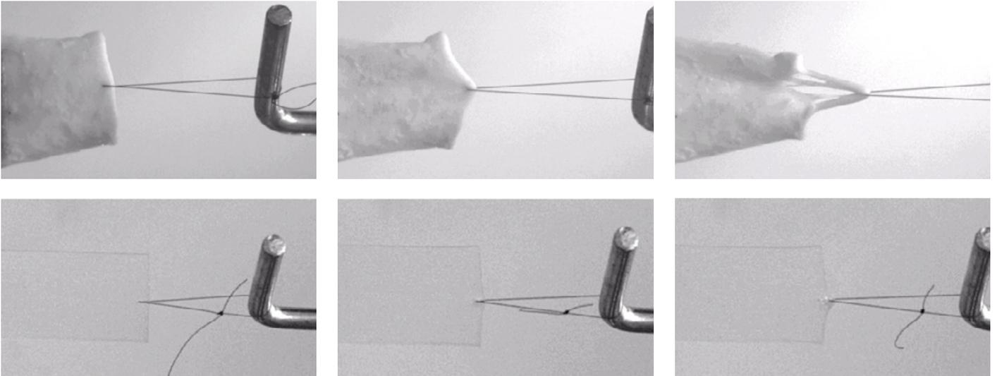
Figure 1: Comparison between single stitch mechanical tests performed on porcine aorta (up) and on a 3DP material (down).
