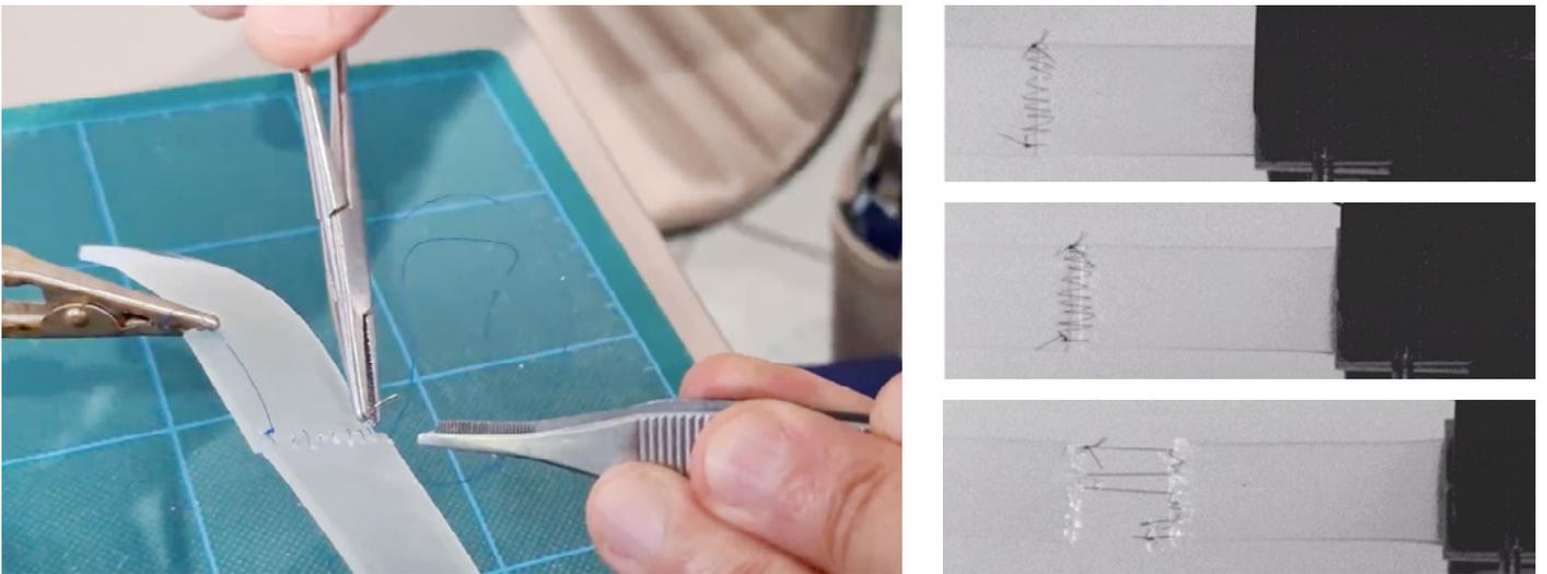
Figure 2: Uniaxial tensile test performed on a 3D printed sample sutured by an expert surgeon in order to mimic the surgical suture on a medium caliper arterial vessel
