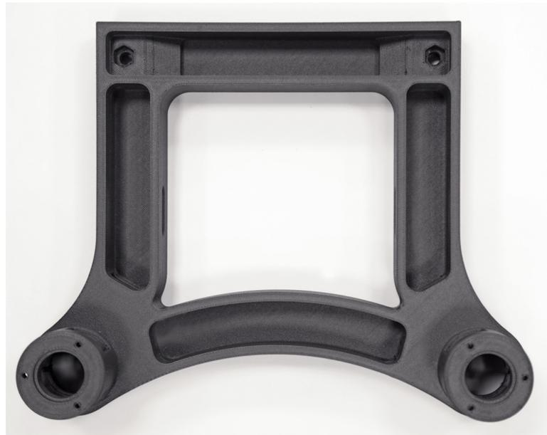
3D printed component used for product handling on the robotic packaging system. Produced using FDM Nylon 12CF material.
