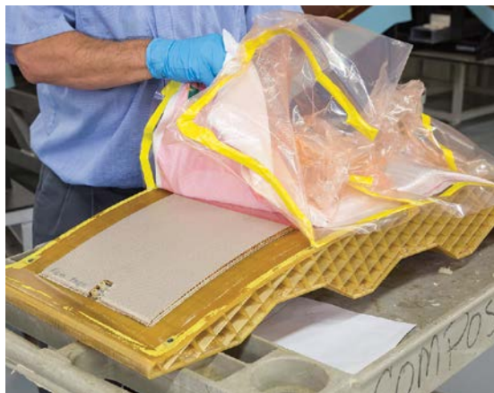
Unbagging the composite lay-up on the ULTEM 1010 tool.
