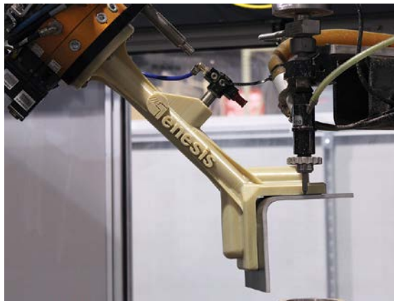
The ULTEM 9085 gripper resulted in a much lighter tool that was much faster to produce.
