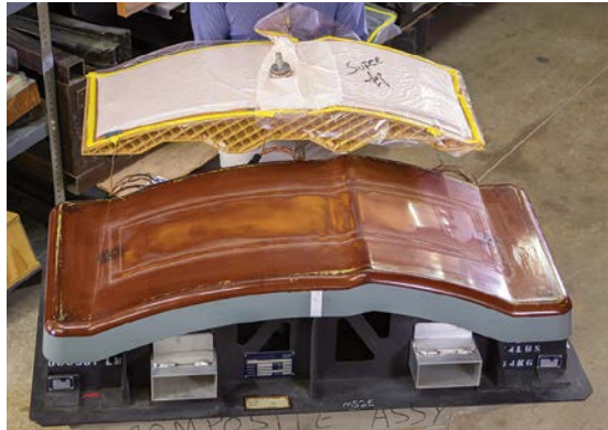
The lighter, FDM tool is shown in the upper portion of the photo compared with the typical FRP tool shown below.
