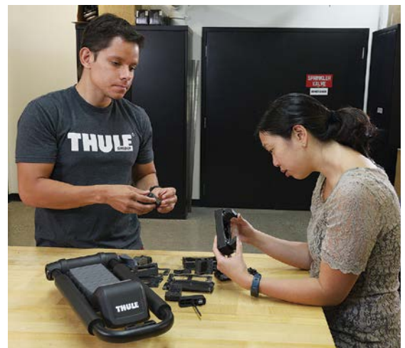
Thule engineers use FDM Nylon 12CF (carbon fiber) material to create functional prototypes.
