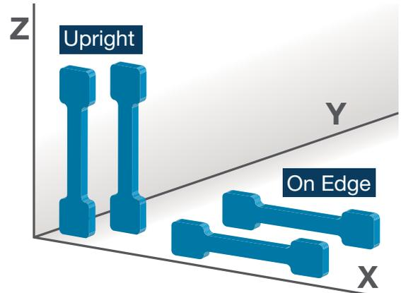
Figure 1: Test sample orientations
