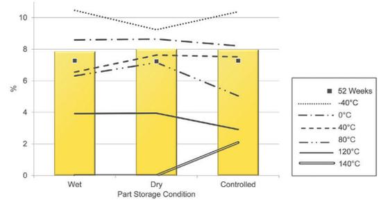
Figure 10a: Elongation at break - 4 weeks, controlled environment, on edge.
