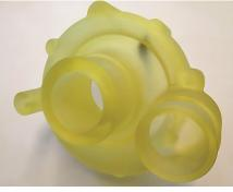
VCE 3D printed this water pump housing in Transparent material for quick functional testing.
