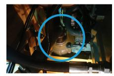
Water pump installed in an A30G for functional testing.
