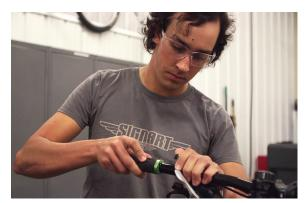
Trek engineering tech Patrick Zeigle mounts a multi-material 3D printed grip onto a bike for testing.
