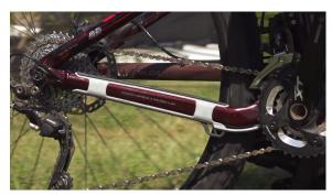
Trek's Objet500 Connex3 created this durable Digital ABS chain guard with rubber-like components in one print job.
