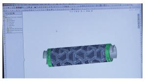
CAD model of an overmolded handlebar grip
