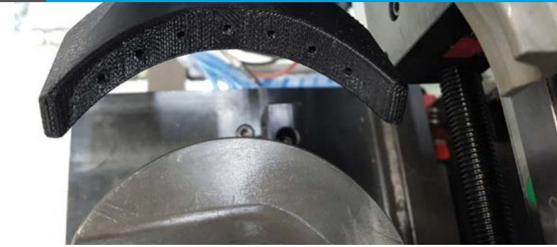
With Stratasys advanced FDM engineering materials, GKN Driveline Florence redesigned a greasing nozzle tool offering improved functionality that helps prevent costly spills.
