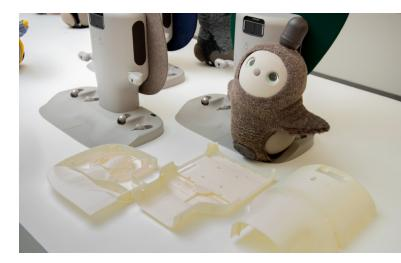
Not only LOVOT's main unit, but also its larger charger is prototyped by a 3D printer.
