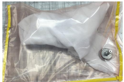
Figure 8-2: Envelope bagging is commonly used with FDM sacrificial tooling.
