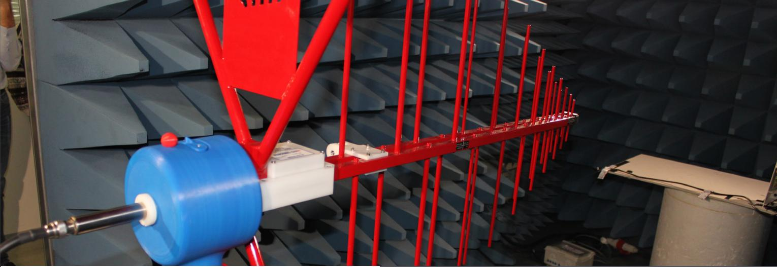
Rotating support for a Bluetooth-testing antenna 3D printed using the Fortus 380mc.
