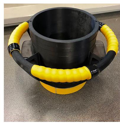
Final, 3D printed ECS duct adapter designed to cool aircraft while on the ground. 3D printed in Stratasys FDM Nylon 12 on the Fortus 450mc.
