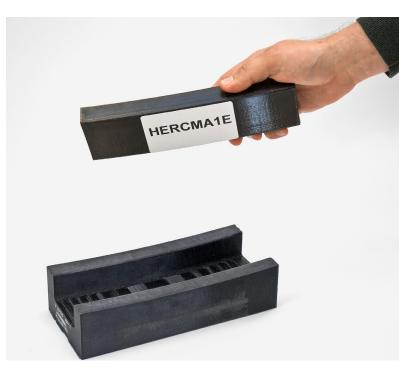
3D printed forming tool in Stratasys Nylon 12.
