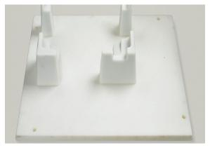
The custom assembly pallets consist of four plastic posts on a Bosch aluminum pallet base. The unit with plastic base shown here is used as a backup.
