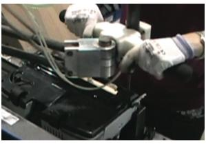
The bottom cover is then positioned and fastened down.
