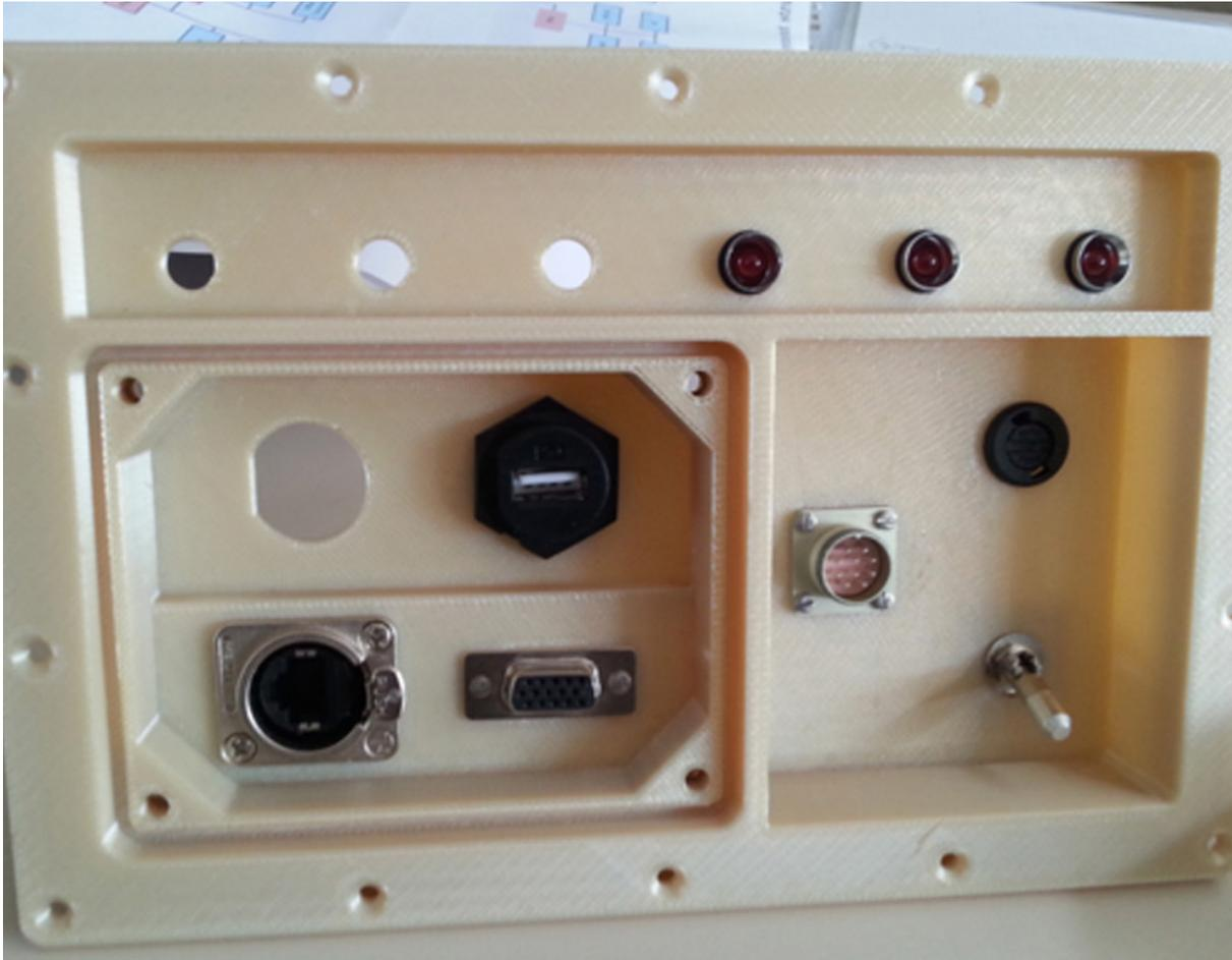
A part of Mini-EUSO produced in ULTEM™ 9085 resin by the team at Laboratori Nazionali di Frascati using its Stratasys Fortus 450mc 3D printer.
