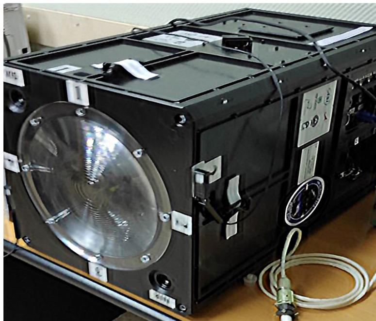
The structure of the Mini-EUSO Flight Model was 3D printed using ULTEM™ 9085 resin on a Fortus 450mc 3D printer.
