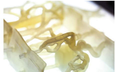
3D printed models based on actual patient CT scans, used both for pre-surgical planning and medical device testing.
