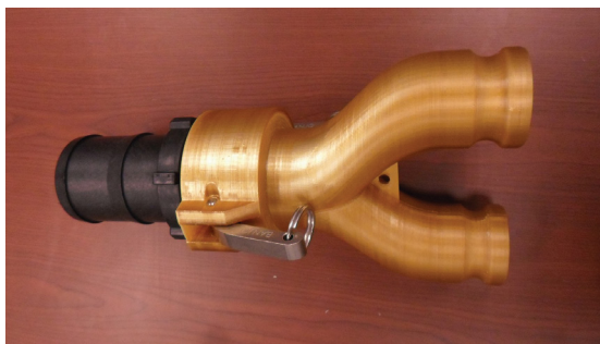
UTC Aerostructures designed a new fume collector for their facility using 3D printed ULTEM 1010 resin material.
