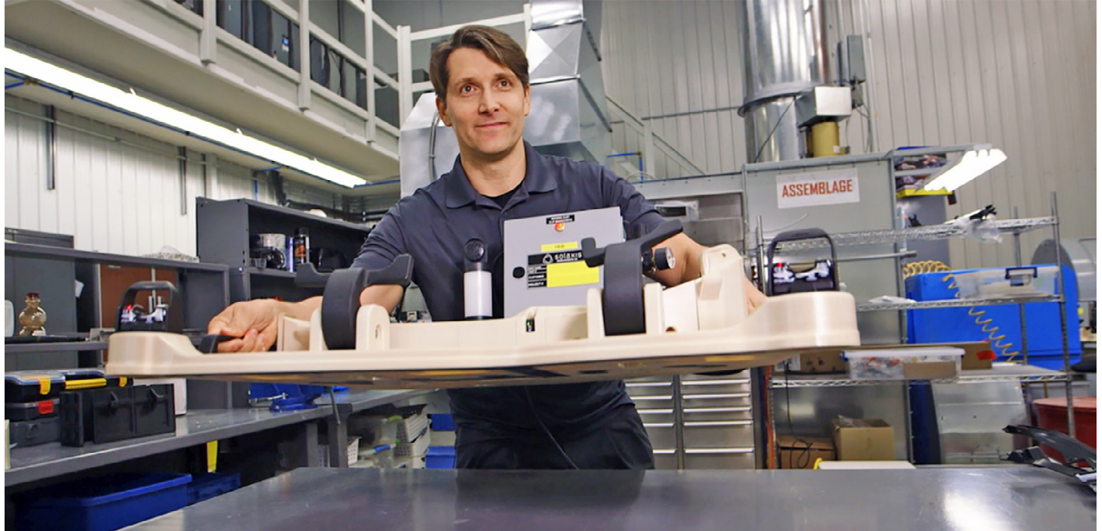
Solaxis president Francois Guilbault demonstrates the lightweight assembly jig produced with FDM technology.
