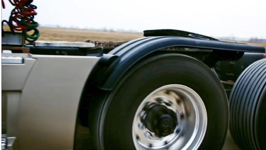
Minimizer put their ULTEM 9085 resin material prototype fenders through real-world functional testing.
